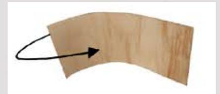
*Husky Form* long grain can be bent in the direction of the length.
